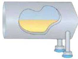
Example 1: The vessel is lifted at one side only. The resulting inclination is small enough not to disturb the readings.
