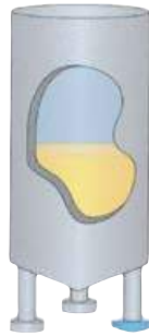
Example 2: One leg of the vessel is just shortened by an inch. No inclination occurs.
