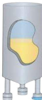
Example 3: The vessel is lifted leg-by-leg, one leg is supported by PanCake. Other legs are leveled out by adding shimming plates.
