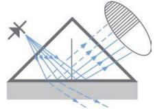
A built-in temperature sensor measures the temperature (T) on the surface of the process liquid. The indicating transmitter converts the refractive index and temperature to concentration units
