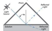
The light source sends light against the interface between a prism and the process solution, where the rays meet the surface at different angles.
