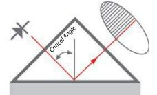
The angle corresponding to the shadow line is called the critical angle of total reflection. This angle is a function of the refractive index (the concentration of the solution.)
