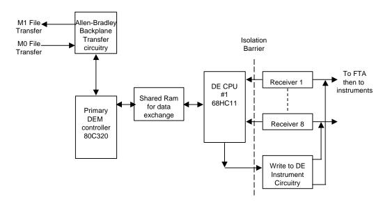
Both Single and/or Multivariable Honeywell Transmitters operating in the DE mode are supported by the module. Supported Honeywell instruments include:
