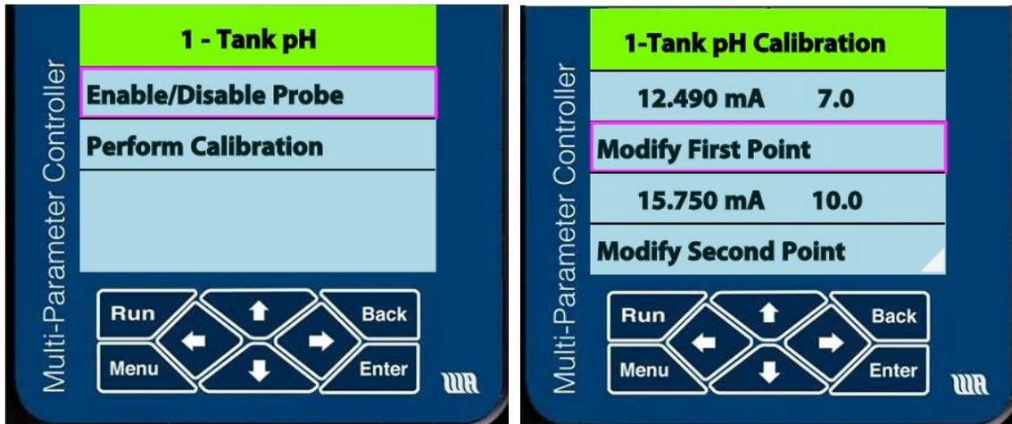
Figure 22- Menu pages for the probe in slot 1, Tank pH, showing the first calibration page.
