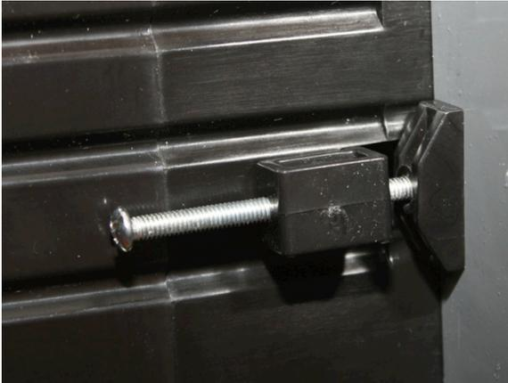
Figure 4 - Mounting hardware attached to panel with 4 in-lb of torque.
