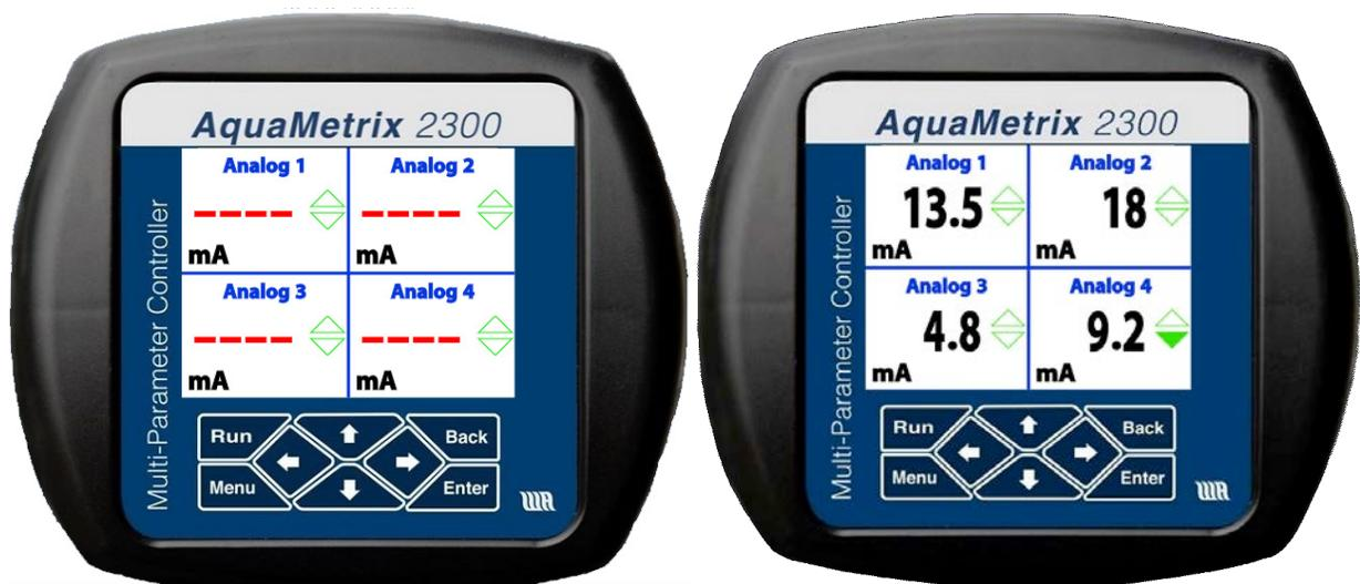
**Figure 4 - The RUN screen showing four analog probe inputs. On the left is a display showing that no probes have been connected. On the right, four analog probes have been connected.**
