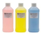
Remember that pH calibration is a two point process involving two of the following calibration solutions: 4, 7 and 10. If your process is on the acid side then you will want pH 4 and 7. If you process is on the caustic side then pH 7 and 10 are the
