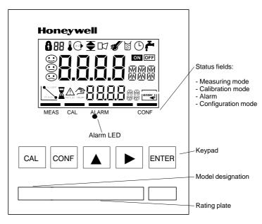
Fig. 10 Front view of Transmitter
