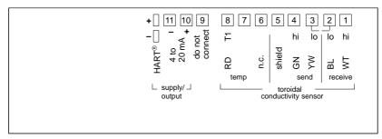
Fig. 7 Terminal assignment of APT2000TC-0(H)-00 Transmitter NI, Class 1, Div 2, Group A – D, T4
