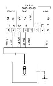
Fig. 9 Conductivity measurement with Honeywell 5000TC toroidal conductivity sensor
