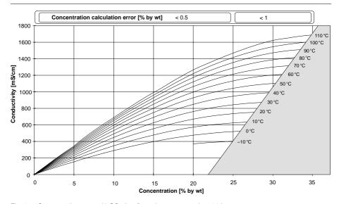
Fig. 15 Concentration curves H<sub>2</sub>SO<sub>4</sub> (configuration: concentration -04-)
