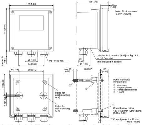
Fig. 2 Dimension drawing for Transmitter, mounting diagram and P/N 51205990-001 panel-mount kit
