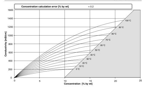
Fig. 14 Concentration curves NaOH (configuration: concentration -03-)
