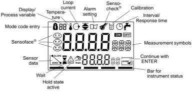
Fig. 11 Display of Transmitter
