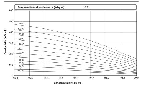
Fig. 17 Concentration curves H<sub>2</sub>SO<sub>4</sub> (range 95 to 99 % by wt), (configuration: concentration -06-)
