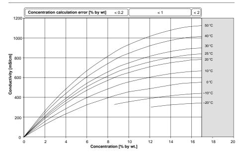
Fig. 13 Concentration curves HCI (configuration: concentration -02-)
