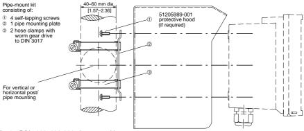
Fig. 3 P/N 51205988-001 pipe-mount kit
