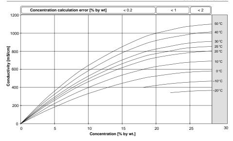
Fig. 16 Concentration curves HNO<sub>3</sub> (configuration: concentration -05-)
