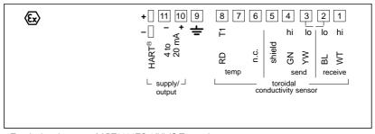
Fig. 8 Terminal assignment of APT2000TC-0(H)-IS Transmitter IS, Class I, Div 1, Group A – D, T4
