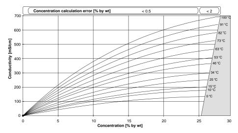
Fig. 12 Concentration curves NaCl (configuration: concentration -01-)
