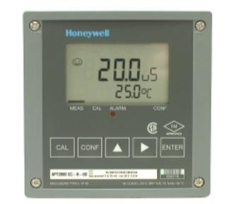
The Honeywell Analytical Process Transmitter (APT) 2000 Series transmitter is a two-wire 24-Volt device that continuously measures conductivity, resistivity and salinity in industrial processes within the power, chemical, pharmaceutical, pulp and paper, and water quality industries.
