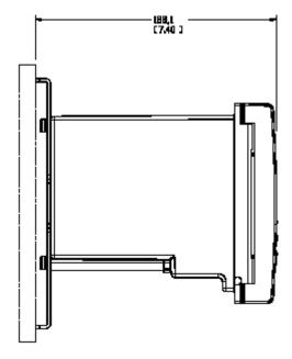
Figure 4 – Wall/Pipe Mounting Dimensions
