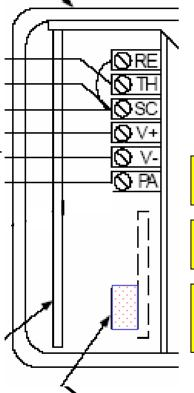
Cable Shield (Yellow) to UDA Chassis Ground Screw
