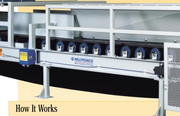
The weigh feeder is used to deliver an accurate mass flow rate of material. The material is profiled by an adjustable mechanical shear gate which fixes the correct material bed depth for a given material particle size.
