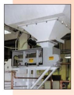
It provides rate and total information and feed rate control functions which help improve product quality and reduce waste. With its precision weigh bridge, the system attains weighing accuracies better than 99.5%.
