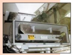
For sanitary applications, a wash down duty motor and gear reducer replace the standard chain driven gear motor. Also, a stainless steel IP67 rated load cell is used to allow the entire unit to be washed down without damage.
