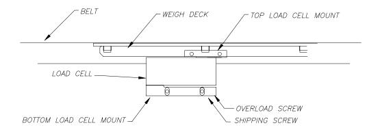
4. Remove the top load cell mount bolts
