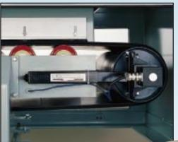
The large diameter 203mm (8") head and tail pulleys allow sufficient surface area to maximize friction at low belt tensions, providing optimum weighing linearity.
