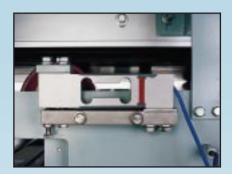
Design features minimize zero drift and allow for the use of very sensitive, precision load cells with very little "dead load".
