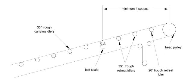
c. On conveyors with 45° trough idlers throughout, a minimum of two 45°, one 35° and one 20° retreat idlers must be located between the scale and the head pulley.
