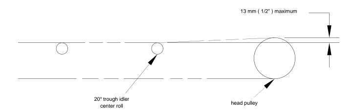
When locating a scale close to the head pulley maintain a maximum of 13 mm (1/2") vertical displacement between the top of the head pulley and the top of the center roll of the adjacent roll.
