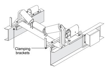
6. The idlers in the weighing area (A2 through R2) must be aligned to and square to the stringers, and levelled to a common reference such as a string or wire (refer to subsequent figures). Ensure that the reference is taut (no sagging). If necessary, shim these idlers to be in line with the reference.
