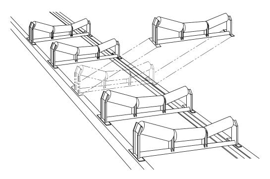
2. Remove the idler foot plates and cut the spine as shown.
