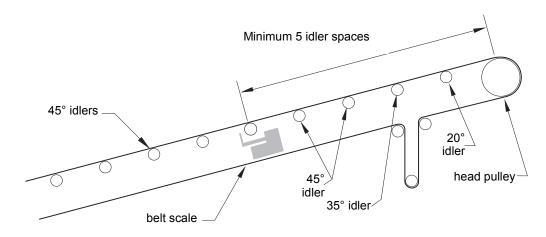
4. The vertical displacement of the head pulley relative to the adjacent retreat idler is normally in excess of that which is acceptable for belt scale installations. It is suggested that when locating the scale close to the head pulley, a maximum of 13mm (½") vertical displacement between the top of the head pulley and the top of the center roll of the adjacent roll be allowed.
