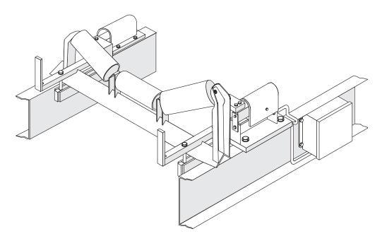
The addition of an idler (supplied and installed by customer) completes the weighing assembly. The MUS load cells provide an electric signal, proportional to load, which is fed to the Milltronics integrator. Thus, weighing occurs without interrupting the process or affecting the process material.
