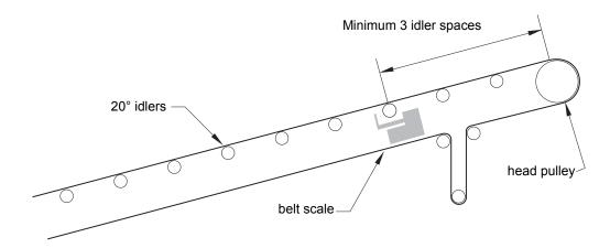
2. On conveyors with 35° trough idlers throughout, a minimum of two 35° and one 20° retreat idlers must be located between the scale and the head pulley.
