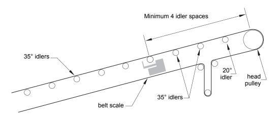
3. On conveyors with 45° trough idlers throughout, a minimum of two 45°, one 35° and one 20° retreat idlers must be located between the scale and the head pulley.
