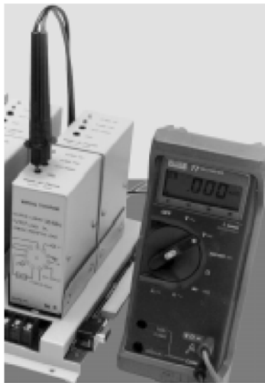
FIGURE 7. Voltmeter Hookup to Measure
