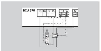
BCU 370 with single-electrode operation, which requires an external ignition transformer TZI or TGI.
