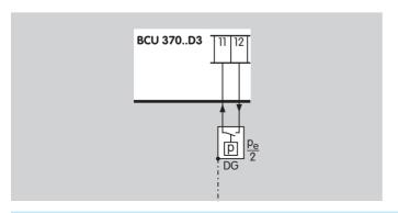
BCU 370..D3, gas pressure switch DG for tightness control
