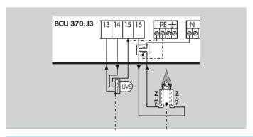
BCU 370...13 for 120 V, ignition by electrode to electrode with centre tap for secondary earthing
