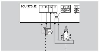
BCU 370..12 for 230 V, ignition by electrode to electrode
