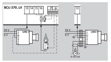
BCU 370..U1 with UV sensor UVD 1 for continuous operation Connection of the 24 V DC power supply with separate wiring in the lower section of the BCU.
