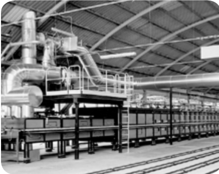
Roller hearth kiln in the ceramics industry
