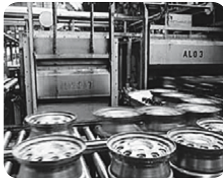
Aluminium industry: curing oven for wheel rims
