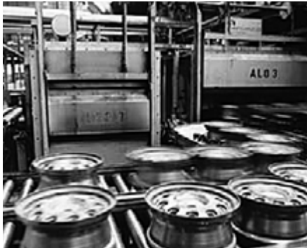
Aluminium industry: curing oven for wheel rims
