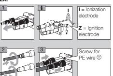
4 Connect the PE wire for burner ground to the fastening lug on the burner insert.
