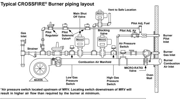
Maxon assumes no responsibility for the use or misuse of the piping layout shown. Specific piping and wiring diagrams should always be sumitted to the appropriate agencies for approval on each application.
