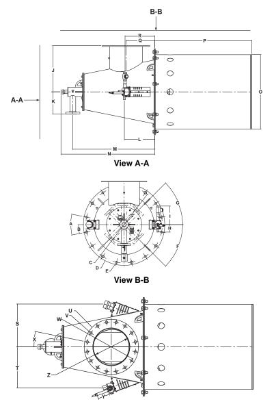
45.5" clearance required to remove burner nozzle
