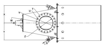
57.5" clearance required to remove burner nozzle
