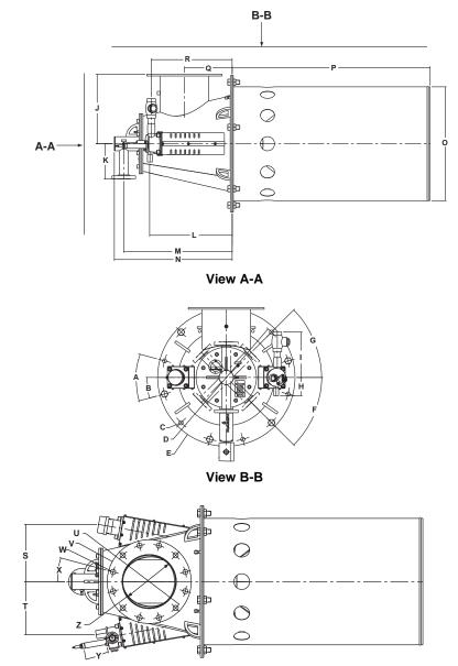
29.5" clearance required to remove burner nozzle
