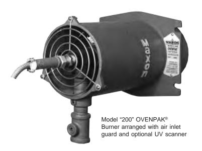
Model "200" OVENPAK® Gas Burners provide a broad range of heat without a combustion blower by firing through-the-wall into your combustion chamber on the suction side of the circulating fan. An internal mixing cone blends air drawn through the burner (by chamber suction) with fuel gas delivered through its central gas nozzle. The Model "200" OVENPAK® Burner is designed for applications involving suction-side firing from -0.2" to -1.6" wc static chamber conditions. They provide:
