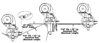
Model "400" OVENPAK® Burner with Control Motor
