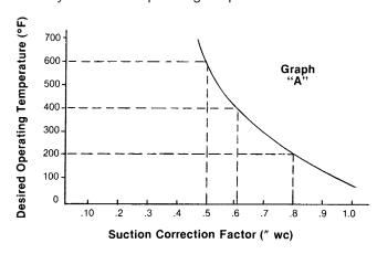
For example, if you anticipate running the system at  $600^{\circ}F$ , follow that dotted line to the right until it intersects curve, then read downward to a correction factor of 0.5. Therefore, if you read a cold suction of 1" wc, your expected suction "at temperature" would be 1" x 0.5 = 0.5" wc.
