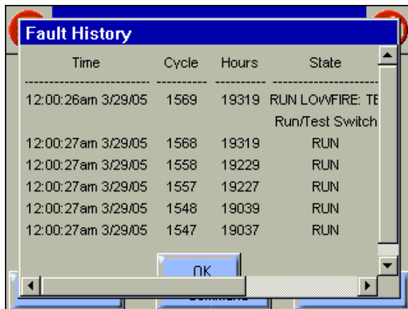
Fig. 63. Burner Control—fault history with time listing.
