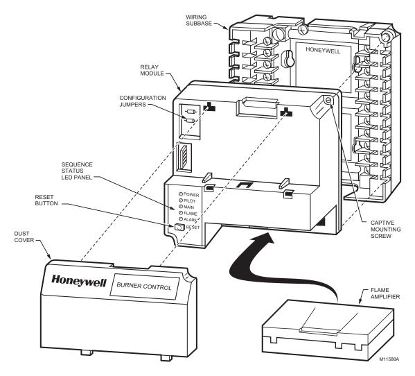
Fig. 4. RM7890 Relay Module exploded view.
