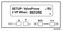
Fig. 8. SETUP: Valve Prove screen.
