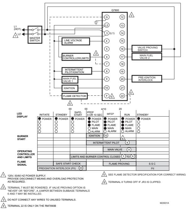
Fig. 3. Wiring subbase and operating sequence chart for RM7890.
