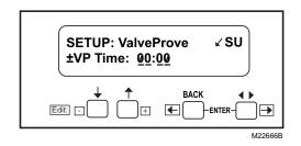
Fig. 10. Valve Prove time screen.
