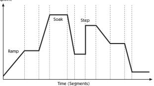
In addition to those settings that determine the segment profile, it is also necessary to set **program start** values, together with the preferred **ramp rate time units** for each individual program.
