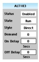
The Alternator is typically used to alternate the starting sequence of a group of pumps, valves, filters, etc. Each block accepts up to 16 inputs and controls up to 16 outputs.
