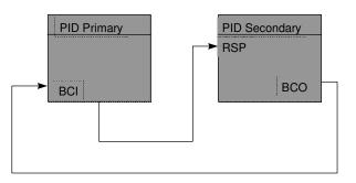
When PID Secondary is in Manual or when Local Setpoint is selected, PID Primary mode is IMAN. IMAN causes the PID Primary output to track the PID Secondary PV.
