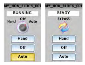
The Hand – Off – Auto (HOA) switch permits state change requests. The block states are: Hand (manual operation from an operator interface), Auto (default – requests are operated automatically), or Off (relay to be switched to Bypass, Hand, or Auto), or Bypass (external manual operation of a device).
