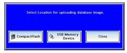
Depending on your device selection, image.sdi file is created on either compact flash or USB memory device. On successful file upload, **Successfully Uploaded Database Image** message is displayed. In case the upload fails, **Error in uploading database image** message is displayed.
