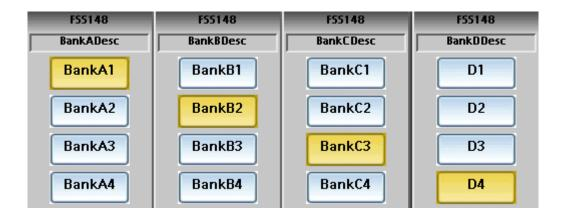
This display has four banks of functions (A, B, C, D). Each function has 4 buttons that act as a 4-position rotary switch, with one and only one state in effect at any time for that function.
