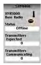
This read-only widget allows the HC900 controller to act as a Modbus master device and communicate with XYR5000 base radios via the serial port of the controller. For attached transmitters there is a separate XYR5000 transmitter widget which is connected to the base radio block via the address output.
