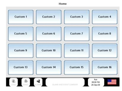
After connecting the Controller and Control Station and downloading your .sds file to the Control Station, the Home display appears with 16 buttons. (Actual button text may vary.)
