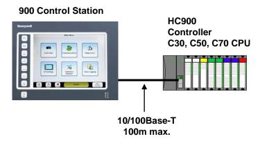
Use shielded CAT5 cable with RJ45 connectors. Connect to HC900 Ethernet port. (On models C70 and C70R with two ports E1 and E2; either port can be used.)
