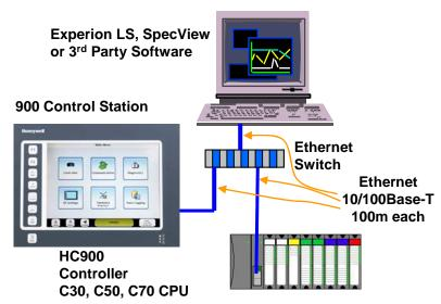
Use shielded CAT5 cable with RJ45 connectors. Connect to HC900 Ethernet port. (On models C70 and C70R with two ports E1 and E2; either port can be used.)
