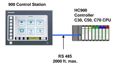
Connect to HC900 RS485 port with unterminated switch settings. S2 port is RS485 terminated by default; S1 port can be configured as RS485.
