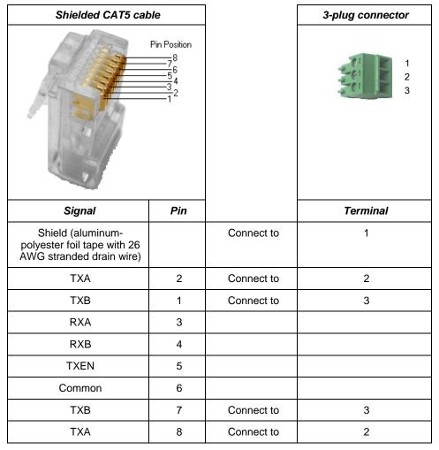
3. Cut off any unused wires in the cable and insulate with heat shrink tubing or other appropriate insulating material.
