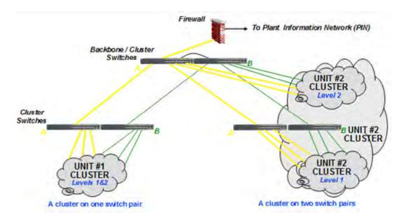
Figure 2 - Basic FTE Network Architecture
