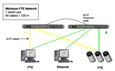
Any of the switch types can be used in the backbone role (top level switches with crossover cables). However, it's highly recommended that the EA-SWHWX1-CN switch be used because it offers an integrated firewall for maximum protection.
