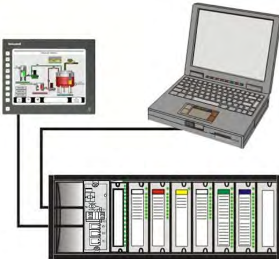
Figure 1 – Small HC900 Controller Configuration
