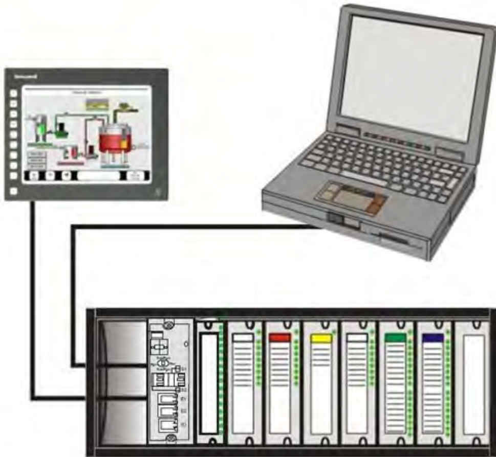
Figure 1 – Small HC900 Controller Configuration
