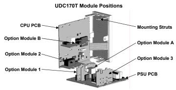
To access modules 1, A or B, first detach the PSU and CPU boards from the front by lifting first the upper, and then lower mounting struts. Gently separate the boards.
