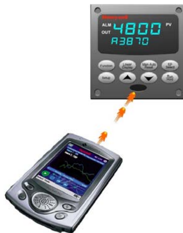
Figure 1-3 Depiction of infrared communications
