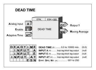
Input E asserted high (1) will enable the operation of the DTM block. When this input is not configured, it will be set high. A low (0) input will cause all registers and the outputs to equal the input A.
