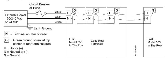
FIGURE 8-28 Daisy Chained Power Wiring
