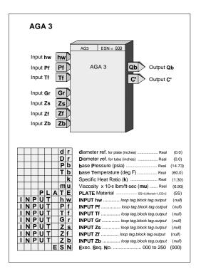
Output  $Q_b$  is updated every scan cycle. Output C' is updated continuously for temperature effects and periodically for other effects. The following conditions are considered in the calculations:
