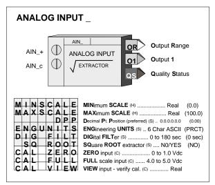
Analog Input blocks are available on the MPU Controller Board (CB) and on the I/O Expander Board (EB). Block names (IDs) are listed in Section 8.4 together with the case rear terminal numbers. Power for 2-wire transmitters is available at the rear terminals.
