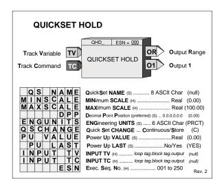
Firmware 1.30 added parameter QSCHANGE. It enables the block output to either update continuously in the Quickset mode as the pulser knob is turned or to only update the output with the value in the numeric display when the STORE button is pressed.
