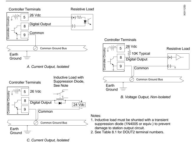
Figure 8-15 Digital Output DOUT1, Resistive and Inductive Loads
