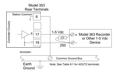
FIGURE 8-13 Analog Output AOUT1, Voltage Output
