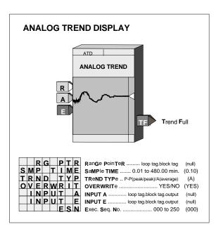
Several inputs can control the operation of the ATD function block. Input E (enable) can be used to enable the trend function when high (1) or unconfigured. Trend action can be disabled by setting E low (0). Each time the function block is enabled a new trend packet will be created.
