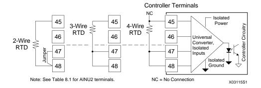
FIGURE 8-18 Universal Analog Input AINU1; 2, 3, and 4-Wire RTD Inputs
