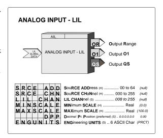
The AIL function can be assigned to a single LIL channel. It will then have certain data that will be accessible over the LIL. Parameter 1 is the received data (RD) in the \$80-\$F80 format and will be re-transmitted by this station on the assigned channel. This LIL CHAN parameter can also be set to 0. The controller will still receive global data from the other station but the received data will not be re-transmitted and the other channel data (i.e. MINSCALE, ...) will not be accessible..
