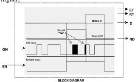
the DLY TIME is adjustable over the full range of the display which is 0.00000 to 999999. In earlier versions, the minimum time setting was 0.1. If the delay time is set to less than the scan time of the station the delay time will equal the scan time.
