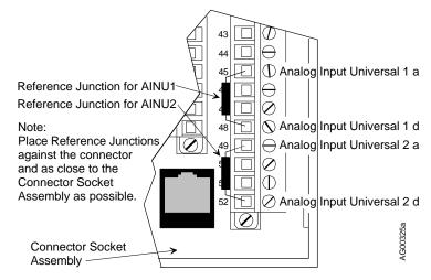
2) Side Entry Connector - Carefully press the reference junction body into the vertical corner, against the Connector Socket Assembly.
