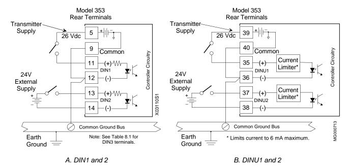
FIGURE 8-14 Digital Inputs DIN and DINU
