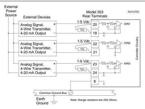
FIGURE 8-10 Analog Inputs AIN1, 2, and 3; 4-Wire Transmitters
