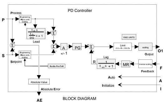
The process range pointer parameter should point to another function block that contains range scaling, such as an analog input that is the source of the process variable. This enables the controller to normalize tuning parameters
