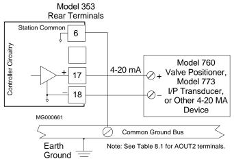
FIGURE 8-12 Analog Output AOUT 1, Current Output
