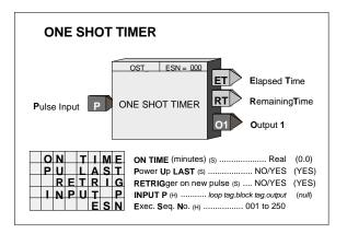
Output ET (elapsed time) will ramp from 0.0 to the value of ON TIME and remain there until P goes low (0). Output RT (remaining time) equals ON TIME - ET.
