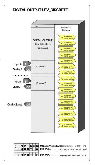
Each function block input also has a quality status associated with it. This status will go high (1) when the block determines it has lost communication with the Lon node bound to that input. If any of the individual quality inputs are high, the Quality Status block output will also be high.
