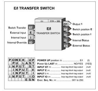
start. During a cold start, it will power up in the position set by the POWER UP parameter. If PU LAST is set to NO, the E/I switch will power up in the last position during a hot start, but during a warm or cold start will power up in the position set by the POWER UP parameter.
