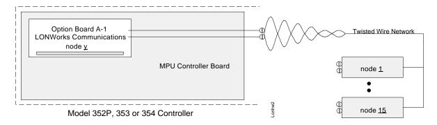
Install a LonWorks network by first wiring all the nodes to the network. Next, temporarily connect a PC-based Network Manager to the network using a SLTA (Serial Link Talk Adapter) manufactured by Echelon Corp. The Network Manager (MetaVision 3.0) and the SLTA are included in the LonWorks Startup Kit.
