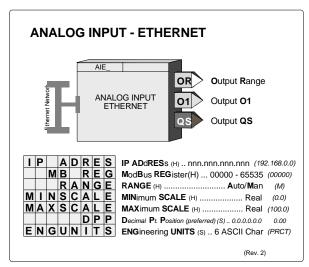
the Modbus Registers from the table below. If this feature is not available, the default setting of the RANGE parameter "MAN" can be used. In this case the range parameters are entered manually. When the auto range feature is used, the range in the AIE block may be out of sync for several seconds if on line changes are made to the AOE range.
