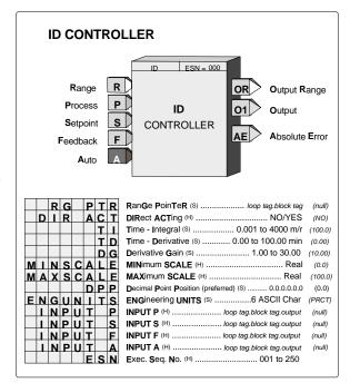
controller to normalize the tuning parameters for the range of the process input. If this parameter is not configured, the controller will use a range scaling of 0.00 - 100.00.
