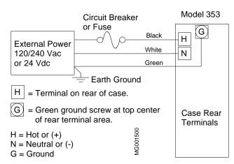
FIGURE 8-27 Suggested Power Wiring
