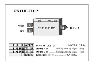
POWER UP - During a warm start, when PU LAST is set to YES, the block will initialize at the input/output states at the instant power down occurred. A cold start will initialize the input/output states to 0.
