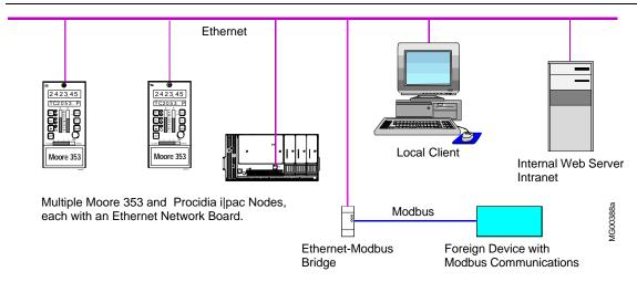
FIGURE 1-2 Ethernet Architecture Example
