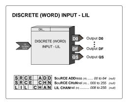
The received global word will also be re-transmitted by this station as a parameter 1 value in the configured channel n.
