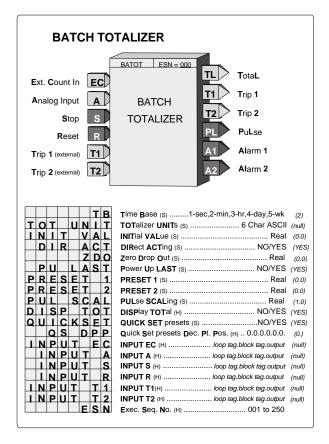
ZDO is used for setting a small positive value, insuring that the integrator will stop when the flow is shut off, which might not otherwise happen if a flowmeter zero is out of calibration.
