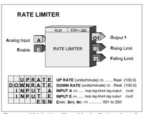
Input E asserted high (1) will enable the limit action of the block. When input E is low (0), the output will track the analog input. If input E is not configured, the limit action of the block will be enabled
