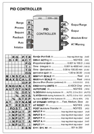
POWER UP - During a warm or cold power up, the output will be initialized to MINSCALE and all dynamic elements will be initialized at the current input on the first scan.
