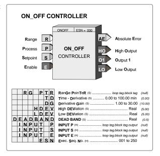
Input E asserted high (1) will enable the block outputs; when low (0) all outputs will be set low (0).
