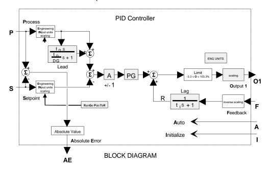
The controller output has MINSCALE and MAXSCALE parameters allowing the output signal to be scaled for engineering ranges other than the default of 0-100 PRCT. This may be necessary when the controller output is the setpoint to another controller.
