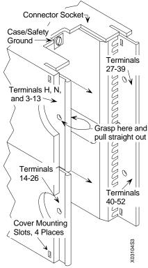
FIGURE 8-2 Side Entry Connectors, Removing a Connector
