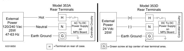
FIGURE 8-26 Controller Power Wiring
