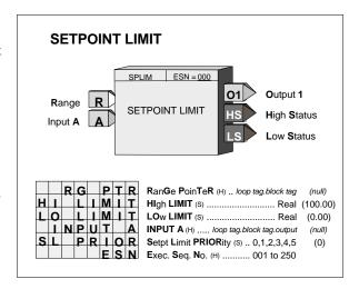
The SPLIM function block has an RG PTR parameter (input R) that defines the normal operating range of the block. Limit settings can be made within -10% to 110% of the range pointer values. If the range pointer is not configured, a range of 0.0 to 100.0 will be used. If a range change is made the current limit value will be moved to be the same % value within the new range.
