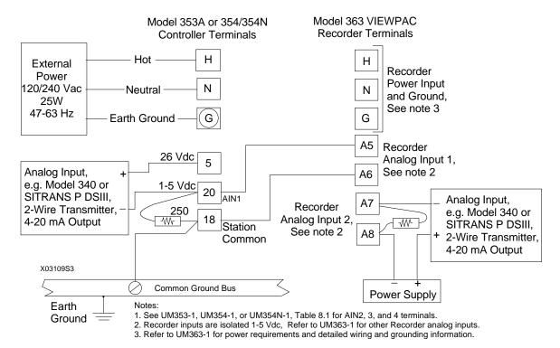
FIGURE 8-25 Moore 353 To Model 363 VIEWPAC Analog Input Wiring
