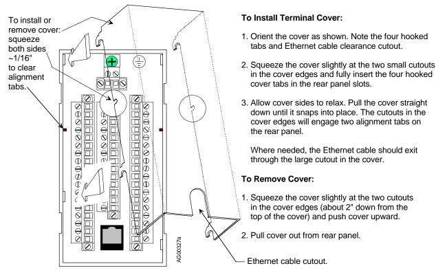
FIGURE 8-1 Direct Entry Connectors, Cover Installation and Removal
