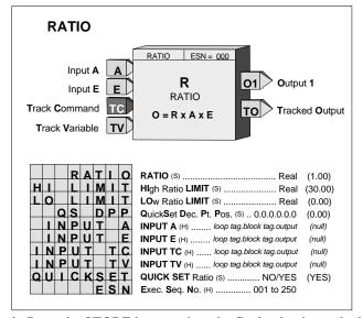
RATIO will continuously change as the knob is adjusted. Press the STORE button when the final value is reached to insure that the new RATIO setting will be retained on a Cold power up condition. The QS DPP parameter enables setting of the Ratio adjustment resolution when in the QUICKSET mode.
