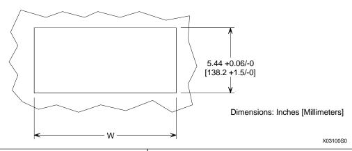
Panel Cutout Dimensions: Tolerances +0.06/-0 [+1.5/-0] Height= 5.44 [138.2] Width= (2.84 X A) + (5.67 X B) - 0.16 inches [(72.0 X A) + (144 X B) - 4.1] mm
