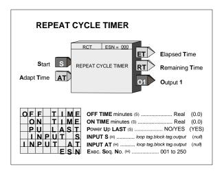
Input S, asserted high (1), will cause the RCT block to start the timing cycle. Output O1 will first go high (1) for a time set by ON TIME and then it will go low (0) for a time set by OFF TIME. It will continue to repeat this cycle until input S is asserted low (0) which forces O1 low (0) and ends the timing cycle.
