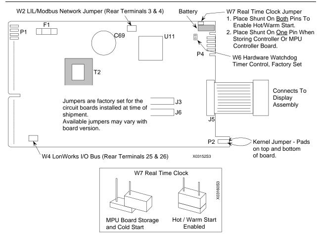
FIGURE 11-3 MPU Controller Board with RTC Jumper W7
