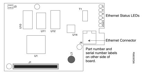
Install the Ethernet board on an MPU Controller board that has a lithium battery that lays against the board.
