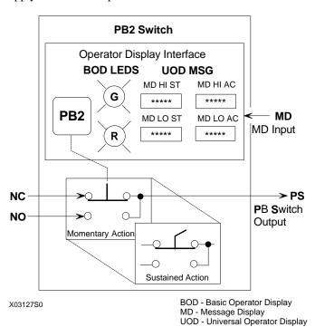
momentary action, it will always power up in the NC position. For sustained action, with the POWER UP parameter set to YES, the switch will power up in the last position during a hot or warm start, and during a cold start will power up in the NC position. When the POWER UP parameter is set to NO, the switch will power up in the last position during a hot start. During a warm or cold start, it will power up in the NC position.
