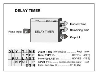
In firmware 1.30 and higher, the DLY TIME is adjustable over the full range of the display, which is 0.00000 to 999999. In earlier versions, the minimum time setting is 0.1. If the delay time is set to less than the scan time of the station, the delay time will equal the scan time.
