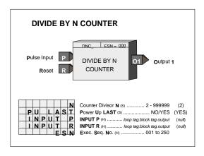
POWER UP - During a hot or a warm start, with PU LAST set to YES, the block will retain the last count and continue at the last input/output states. If set to NO, during a warm or a cold start, the output and count will be initialized to 0.
