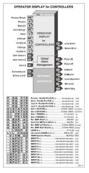
Input variables P, S, V, X, and Y are shown in the numeric display, using the engineering UNITS and the preferred DPP of the range pointer. The Total from the BATOT will also be displayed when configured within the BATOT block. If a value is greater than allowed by the DPP parameter, the decimal point will be shifted to allow the display to show the full number, until it exceeds the maximum available digits, at which time it will indicate over range.
