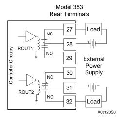
FIGURE 8-21 Universal Relay Outputs ROUT1 and 2, Resistive Load
