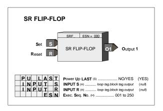
POWER UP - During a warm start, when PU LAST is set to YES, the block will initialize at the input/output states at the instant power down occurred. A cold start will initialize the input/output states to 0.
