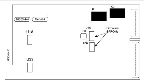
FIGURE 11-4 I/O Expander Board
