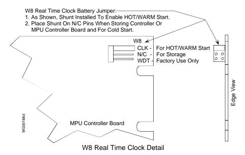
FIGURE 11-2 MPU Controller Board with RTC Jumper W8
