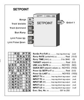
The RG PTR, range pointer, parameter determines the normal operating range of the function block. If the pointer is not configured the block will use 0.00 to 100.00. The range of the setpoint block will be limited to -10% to 110% of the range parameter. If a range change is made the current setpoint, ramp rate, target setpoint, and power up setpoint will be moved to be the same % values within the new range.
