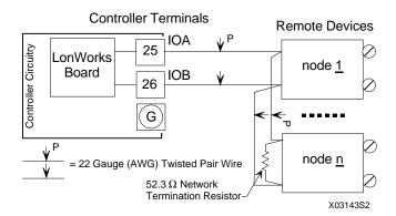
FIGURE 8-23 LonWorks Network Wiring
