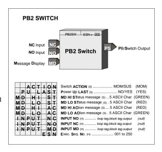
This block operates with an operator faceplate that includes green and red LEDs that are turned on using input MD. A HI (1) input will turn on the Green LED and a LO the Red LED. The default connection will be the PS output of the block but should be changed as required to display the correct status. The message parameters do not apply to the current product.
