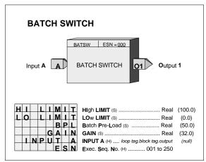
As input A equals or exceeds the HI or LO LIMIT setting, the output of the batch switch will be either decreased (HI LIMIT) or increased (LO LIMIT), changing the feedback signal and therefore the controller reset signal. This maintains controller output at the batch switch limit setting and eliminates reset windup.
