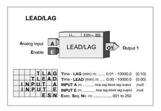
POWER UP - During a warm or cold start, the dynamic elements and the output will be initialized to the value of the current input on the first scan.
