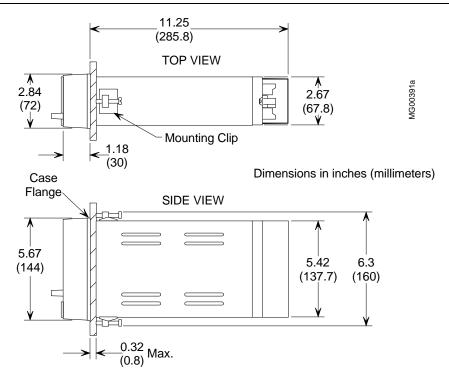
FIGURE 8-4 Moore 353 Dimensions, Direct Entry Connectors
