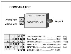
DEAD BAND - the output will return from a high (1) output to a low (0) output when input A is less than the limit - Dead BAND setting for direct action or greater than the limit + Dead BAND for reverse action.
