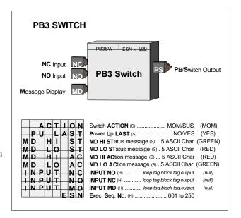
This block operates with an operator faceplate that includes green and red LEDs that are turned on using input MD. A HI (1) input will turn on the Green LED and a LO the Red LED. The default connection will be the PS output of the block but should be changed as required to display the correct status. The message parameters do not apply to the current product.
