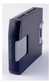
Each Single Loop Module is an independent PID controller. Up to a max of eight Loop Modules can be connected to a single Bus Module. Each Loop Module contains its own PID processor as well as all input and output connections. Mixed installations of Single and Multiple Loop Modules are possible. Each Loop Module can be removed and replaced (Hot Swapped) whilst the process is running.
