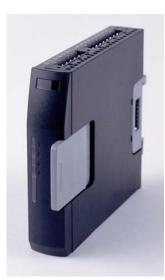
Each Three Loop + Heater Break Module is an independent PID controller with 3 loops of control and heater break detection input. Up to a maximum of eight Loop Modules can be configured for each Bus Module meaning it's possible to have 24 loops of control all with Heater Break detection. Mixed installations of Single, Three and Four Loop Modules are possible. Each Loop Module can be removed and replaced (Hot Swapped) whilst the process is running.
