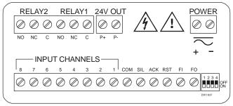
Figure 2. Connector Labeling for PD158-6R2-1
