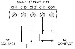
Figure 4. NO/NC Contact Inputs
