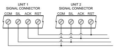
Figure 11. Shared Pushbutton Connections
