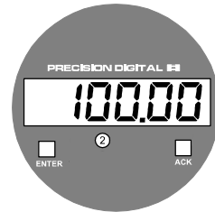
Meter displaying preset for set point 2
