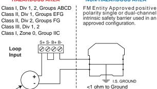
FM Entity Approved transmitter installed per transmitter manufacturer's Hazardous Location Installation Drawing.
