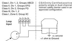
CSA Entity Certified transmitter installed per transmitter manufacturer's Hazardous Location Installation Drawing.
