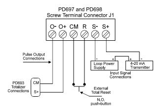
NOTE: When using a four-wire connect the transmitter's positive terminal to S+ and the negative to S-
