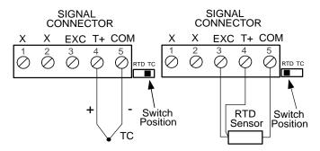
Thermocouple and RTD Inputs
