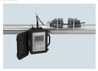
SITRANS FUP1010 clamp-on non-intrusive ultrasonic flow transmitter offers maximum versatility plus battery power for portable field use. It can operate in either WideBeam transit time or reflexor (Doppler) mode, making it suitable for virtually any liquid, even those with high aeration or suspended solids.
