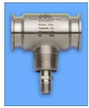
**Note:** Turbine meter must be installed with pickup coil pointing down to ensure proper cleanability according to the 3A standard.
