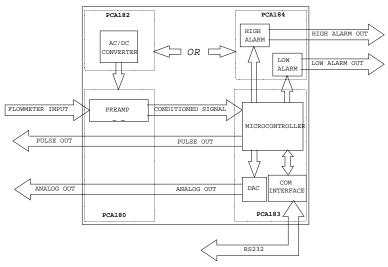
An RS232 communications port located under the top plate allows CAT3 to be remotely configured using a Windows based application that included with all units. Configuration and remote monitoring may also be performed using any PC based communications program (e.g., HyperTerminal) or ASCII terminal.
