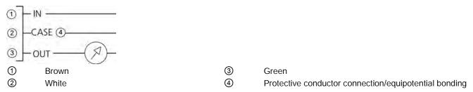
Figure 5-2 Pressure transmitter, electrical connection
