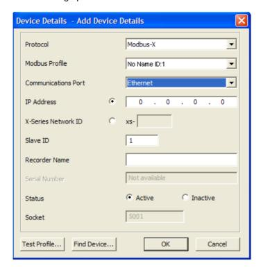
The Protocol should be matched to that set on the recorder. It will be Modbus-X by default so leave it at that unless you changed it on the recorder.
