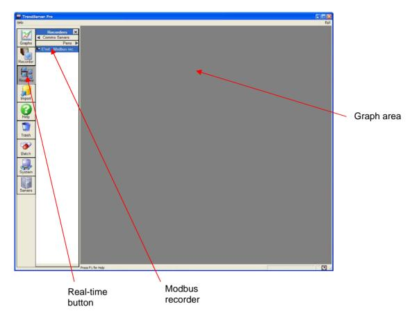
Either click and drag the recorder name from the list to the graph area, this will add all the recorders pens onto the graph, or click on "pens", to list the pens available and drag the pens onto the graph.
