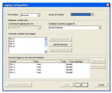
Drop down the "Device ID Number" list and select the recorder from the list.
