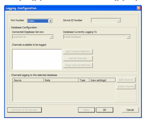
Change the "Port Number" to Ethernet (or the correct port if using RS-485). This will allow access to the other dialog boxes.
