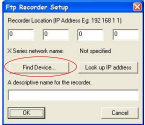
Press the "Find Device" button. This will cause Trend Server to go and check the network for recorders. It will give a list of all the recorders it can find, listing Recorder Name (the recorder name shown in the top right hand corner of the recorder screen), network name (xs-nnnnnn, where nnnnnn is the recorder's serial number) and IP address.
