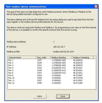
When every thing has been entered use the "Test" button to make sure that everything is set up correctly.
