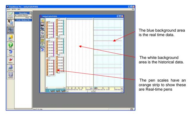
The white area for historical data will display the data that is stored to the database. At this point we have no data being stored to the database, it is simply being acquired and graphed, and if the graph is closed any data downloaded via Modbus will be lost.
