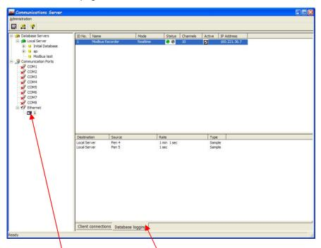
The screen should now show the pens logging for that recorder and their log rate. In this case 2 channels are logging at different rates, one every second and one every 1 minute, 1 second.
