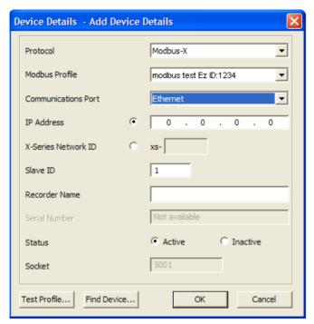
Enter the IP address that was noted during recorder set up or enter the Network ID for X Series recorders only; this is the recorder's serial number. Eq. xs-999999.
