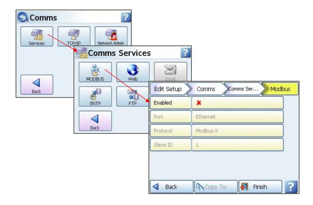
Hit the "Enable" button to enable Modbus. Leave the Port and Protocol as default. Enter a slave ID number.
