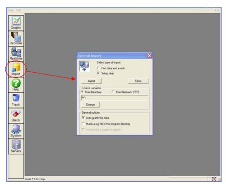
When the External Import box appears select "Setup only" and use the "Change" button to browse for the device location.
