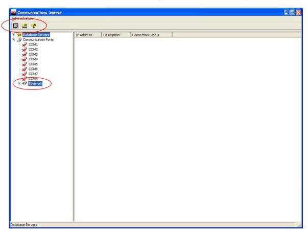
For connection via ethernet. Double click the ethernet icon in the left column. This will activate ethernet, the red cross will change to a black tick.
