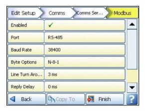
The Slave ID must be set; this is used by the PC to identify recorders. Each recorder must have a different slave ID.
