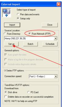
Or for Ethernet connections the setup can be downloaded from the recorder via FTP. Select "Setup only" as shown, but change "from directory" to "From Network (FTP)".
