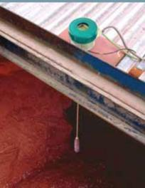
Pointek CLS300 is ideal for harsh process conditions with high chemical and physical demands where reliability and accuracy are critical for safe and economical operation. It is used for high and low level alarm, or as a back-up for continuous systems in high pressure and temperature applications.
