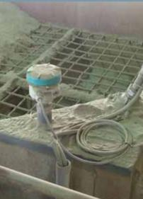
Pointek CLS200 is a versatile level switch ideal for high and low level alarm, or as a back-up for continuous systems of liquids, solids, slurries, foam, pump control, and interfaces in general process conditions with high chemical and physical demands.
