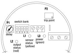
The alarm delay and trip point settings can be adjusted, using indicators L1, L2 and L3 to help set potentiometers P1 and P2.
