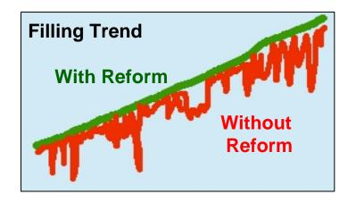
Echo Reform joins echoes together, thus eliminating drift and providing a more accurate and reliable signal.
